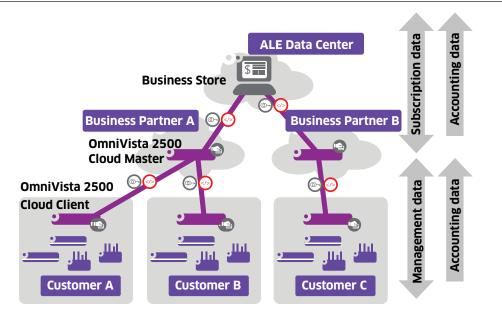
These three zones are interconnected through the Internet, and all connection links are secured with strong encryption, authentication, and access controls. All individual network elements are designed to implement the technical measures described in this document.
